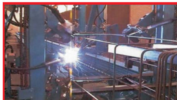
Máquina Cage Master - Progress Maschinen & Automation (Alemanha) - Processo Robô MIG ( www.progress-m.com )
